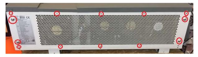
2. Once the screw removed the lateral panel will come off.
