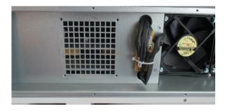
6. Put back the lateral panel and screw the 14 screws.
