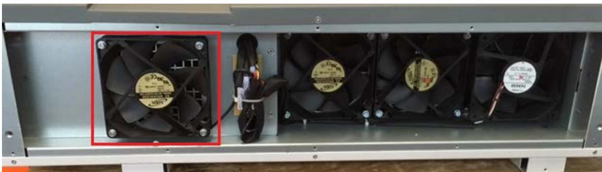
3. Unplug the fan power cable from the connection board. The cable to remove is shown in the below picture (connector in the red square).
